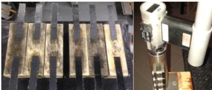
**Fig. 8 DSS-test (Direct Shear test)**
